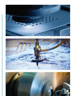
**Cutting Methods** From the top: Laser Cutting, Water-jet Cutting, Mechanical Cutting.
